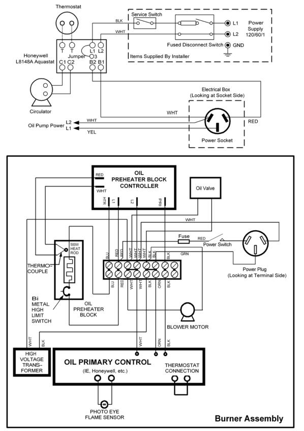
Figure 33. WIRING DIAGRAM, SINGLE HEATING ZONE ONLY
